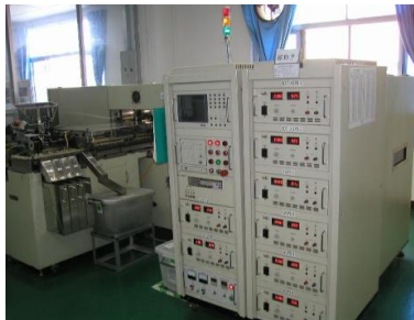
Aging: All Characteristics 100% tested under high temp. & pressure
