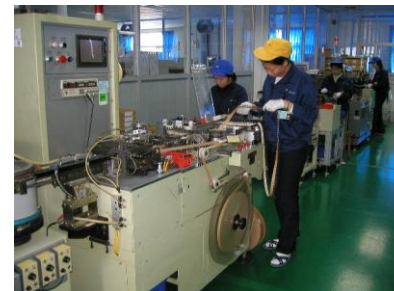
Taping & 100% Characteristics Inspection
